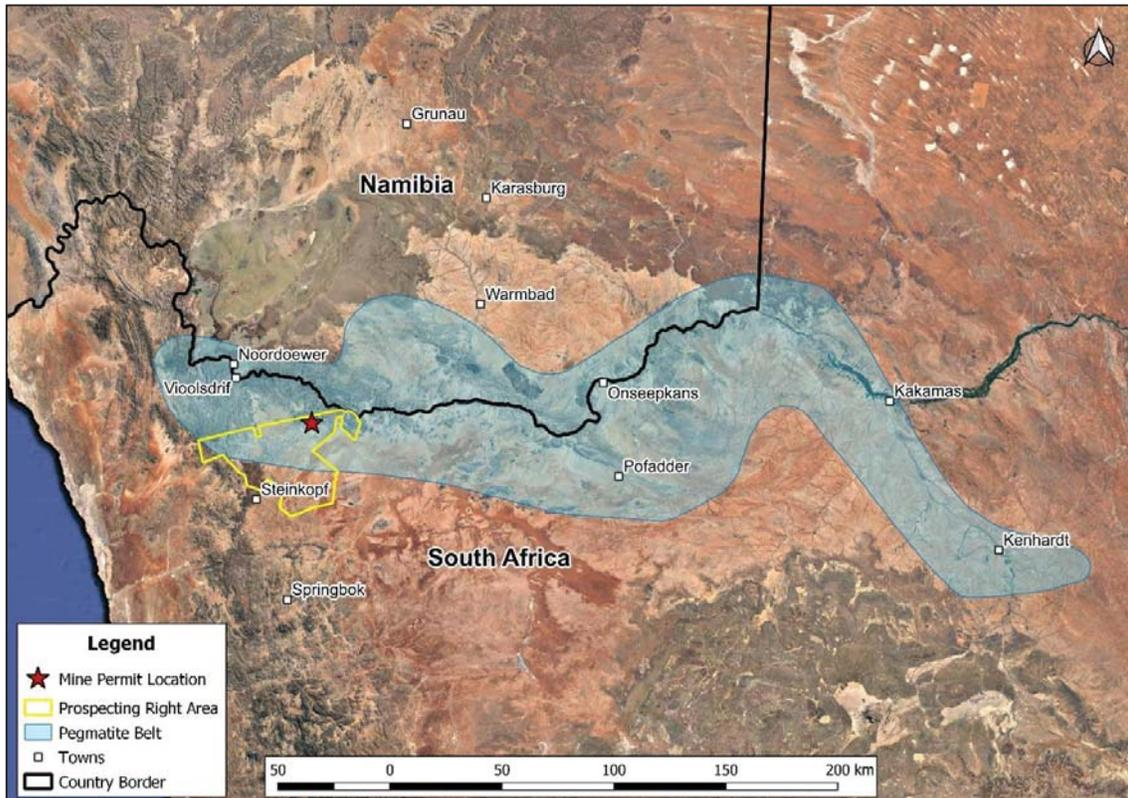
Figure 6: The 16 km wide, ca. 450 km long, pegmatite belt hosted by basement rocks of the Namaqualand Metamorphic complex. The locations of prospecting right and mine permit in relation to the belt are indicated on the map.
