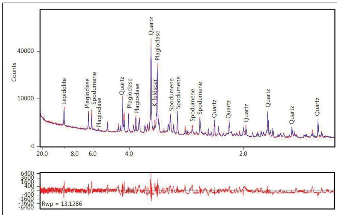
Figure 13: X-ray diffractogram showing the mineral identification for the pegmatite sample. The upper red pattern is the measured diffractogram, the blue pattern is the theoretical diffractogram generated during the refinement and the lower red pattern is the difference plot.
