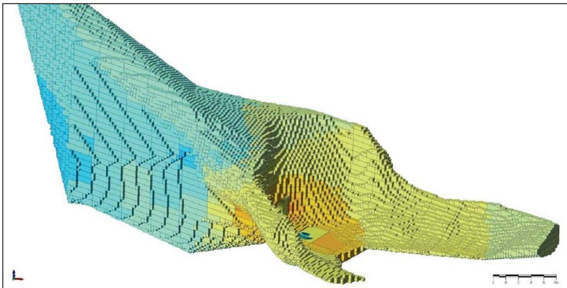
*Figure 18: Li<sub>2</sub>O Block Model.*
