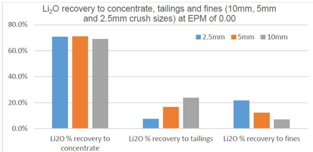
Figure 14:  $\text{Li}_2\text{O}$  recovery to concentrate, tailings and fines at the three crush sizes.
